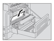
4 Open the transport guide of the paper feeding area and check if any paper is jammed under this guide. Clear the paper if there is any.
